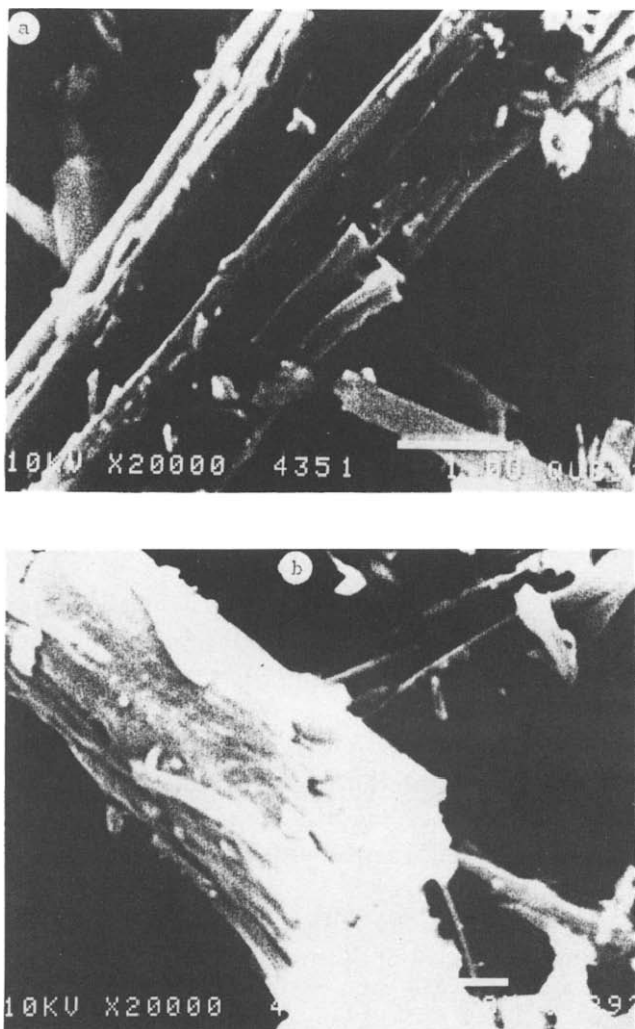
Fig. 9. (a) Scanning electron micrograph of NiODH heated at 320°C. (b) Light crushing of NiODH heated at 320°C revealed an internal slab-like structure.
